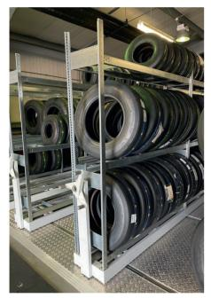
The mobile storage system is designed to provide unsurpassed levels of performance and strength designed for 24/7 repetitive use. The carriages are manufactured from fully welded cold rolled steel which is precision punched and welded in jigs to maintain accuracy. All drive and running gear components are of the highest quality available. All nuts and bolts are nyloc bright zinc plated high tensile grade 8.8.
