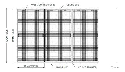
Solution using frames secured into floor and ceiling; for fixing without reinforced walls and extreme heavy duty applications:
