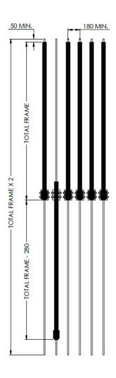
Solution using top guide rail fixed directly into ceiling, for room heights up to 3110mm:
