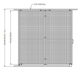
Solution using floating rails for room heights above 3110mm or bespoke applications:
